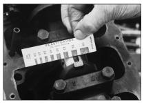
The normal clearance in the big-end or main bearing should be approximately one part in 2,000 of the diameter. Thus a journal of 2" (50.8mm) in diameter may be expected to show a clearance of 0.001" (0.025mm).
