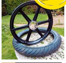
WHEELY LOVELY FINISH STEP I'm really pleased with the satin black powder coating on the wheels. It's tough enough to resist tyre lever damage when fitting the tyres. We've chosen a pair of Avon Roadriders to wrap around them.
