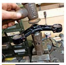
BEARING FALSE START STEP Unless you have a sleeve of exactly the right diameter, fit the outer race to prevent damaging the bearing cage. It all had to come off again, though: I realised the headlight bracket lug is missing ...
