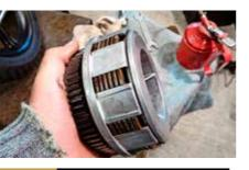
ASSEMBLE THE CLUTCH I found it easiest to assemble the clutch on the bench - plates onto pressure plate, slide the lot into the basket, aligning the external tangs - then fit it as a unit.
