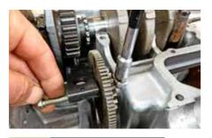
SLIDE IN SELECTOR STEP Slide in the selector drum, retained by an
