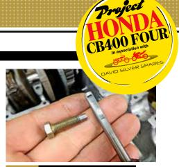
STEI THE TENSION Fit the tensioner and lock it, fully down with the bolt. The bolt must locate the flat on the rod to give the range of movement. Check the bolt locks and releases it.
