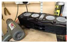
SPRAY THE BARRELS I fitted the old base and head gaskets for masking, using some bolts to locate them and weight them down, then sprayed the barrels satin black to match crankcase.
