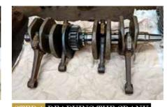
READYING THE CRANK I assembled all the rods onto the journals they came from with a little clean engine oil and torqued down to the setting in the manual leaving the crank ready to fit.
