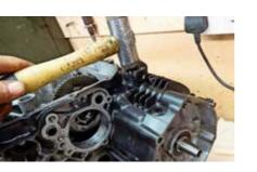
STEP 14 APPLY THE MALLET Tap the cases to seat the dowels, then replace the bolts. Nip up the M8 main bearing bolts lightly with a spanner, then lightly tighten the gearcase bolts topside.
