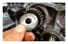
STEP 17 FIT THE PRIMARY GEAR With primary shaft spacer, bearing and circlip installed, fit the primary gear. At least there's no mistaking which way the cupped washer goes; Loctite the bolt.
