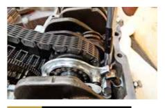
STEP 11 ARE U KEEPING UP? Refit the camchain tensioner U-bracket, Loctiting the bolts. This is an upgraded, machined aluminium reproduction part, available from Dave Silver.
