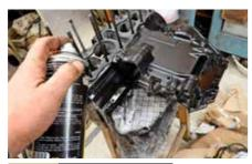
BACK TO BLACK The cases were scruffy and corroded. Vapour blasting is good, but we wanted to stick with black, so I heated the cases and sprayed them with satin case paint.
