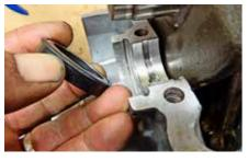
STEP 6 PLATFORM ONE Temporarily replacing the head/barrels provides a platform for the inverted top crankcase. Fit seals either end, both chains, oil shells and lay crank in bearings.
