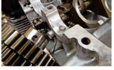
BEARING DOWN STEP You can't shrink-fit bearings into a split crankcase, so the Honda bearings have dowels and half-circlips to retain them and prevent spinning. Carefully locate them.
