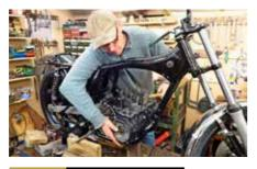
STEP [ BOTTOM END IN I decided now was the time to put the crankcase back in the fame; it was a lot more manageable than when I removed it in one piece and saves chipping the paint.
